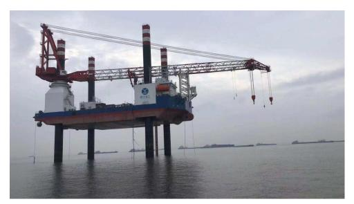
A wind turbine installation vessel can rapidly raise its hull clear of the water to provide a stable platform for offshore construction and O&M works
