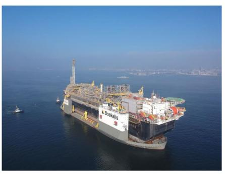
Largest ever cargo transported by a Heavy Transport Vessel at 80,000 MT and 288m length
